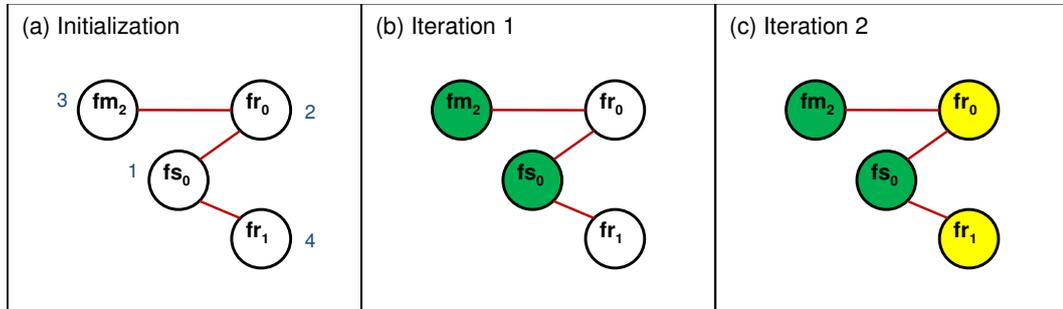
Figure 7.10: Welsh-Powell algorithm for graph coloring
