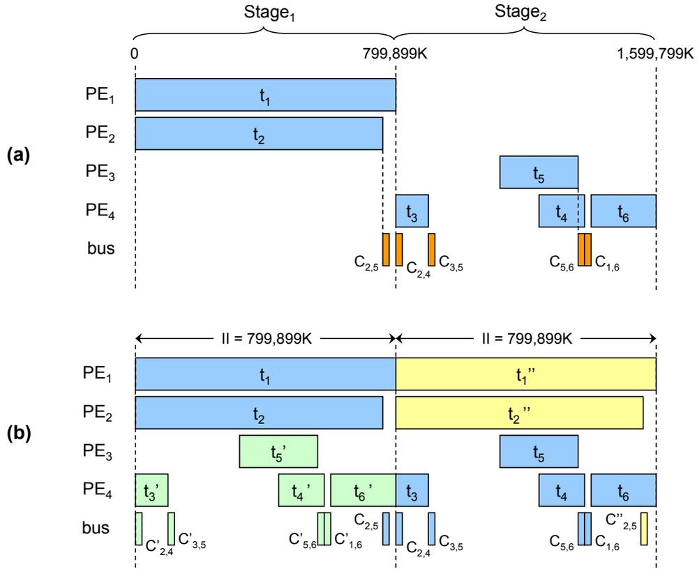
Figure 8.7: An optimal pipelined schedule for the task graph in Figure 8.5 with (a) single-instance execution view, and (b) steady-state execution view
