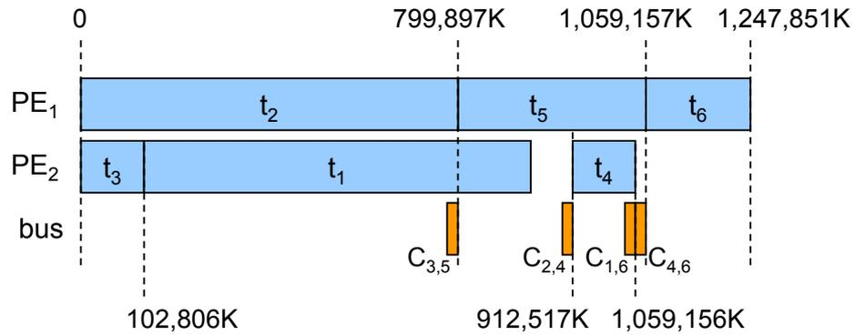
Figure 8.6: An optimal non-pipelined schedule for the task graph in Figure 8.5 on four processors
