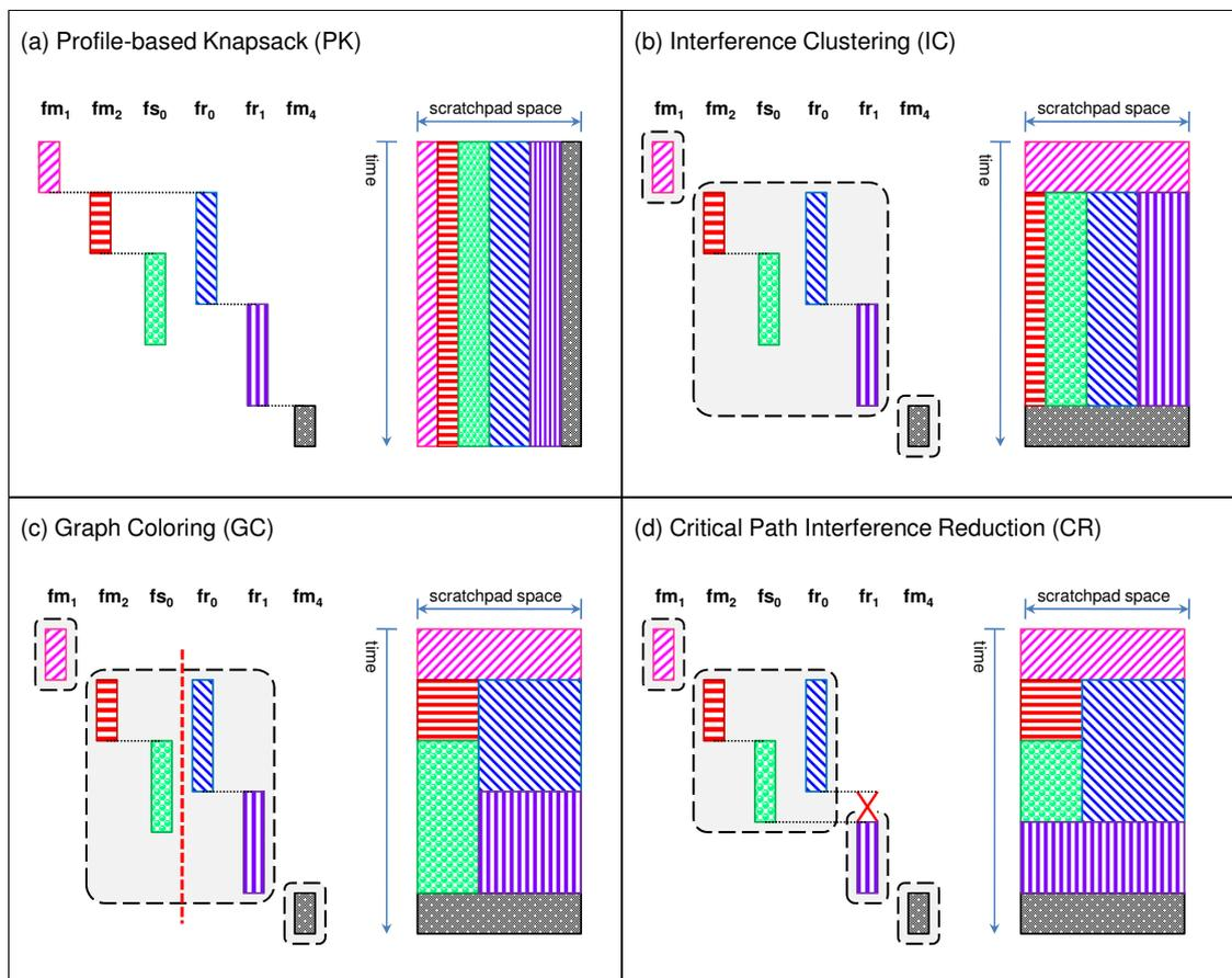
Figure 7.9: Four considered allocation schemes with varying sophistication
