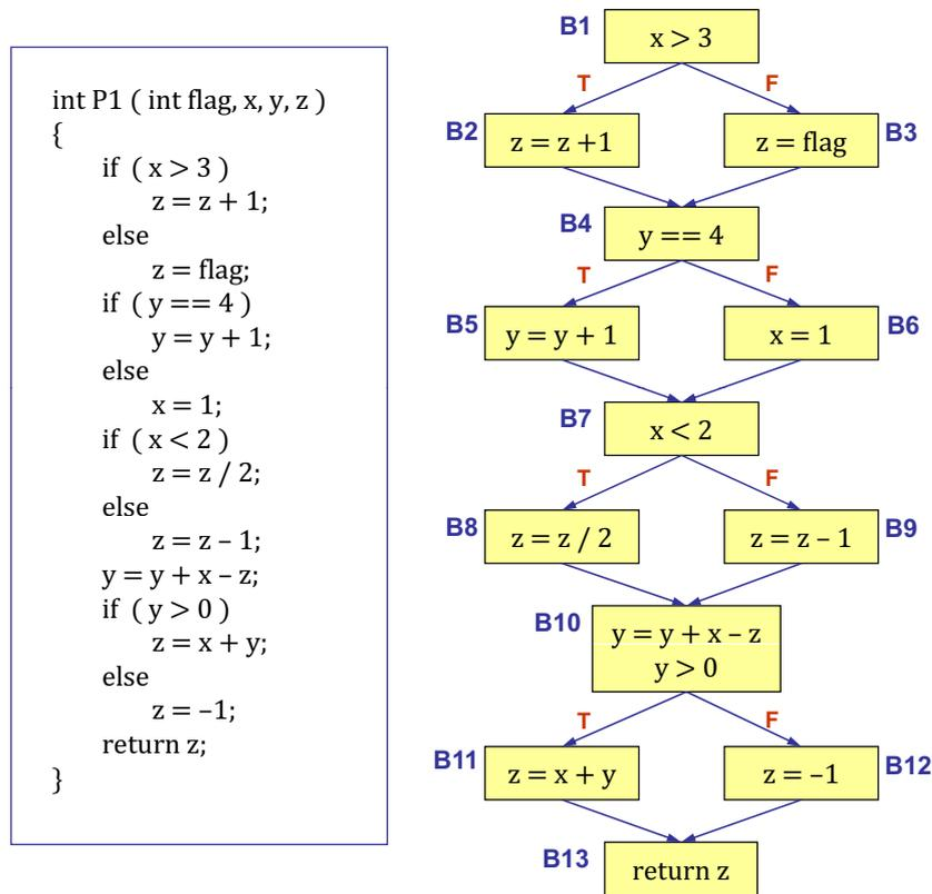
Figure 4.1: An example program and its control flow graph (CFG)
