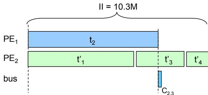
Figure 8.3: Optimal pipelined schedule for the task graph in Figure 8.2 without considering data allocation
