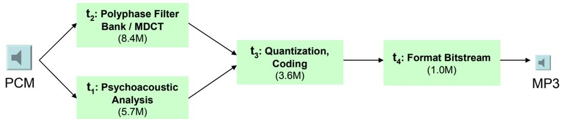
Figure 8.2: Task graph of LAME MP3 encoder
