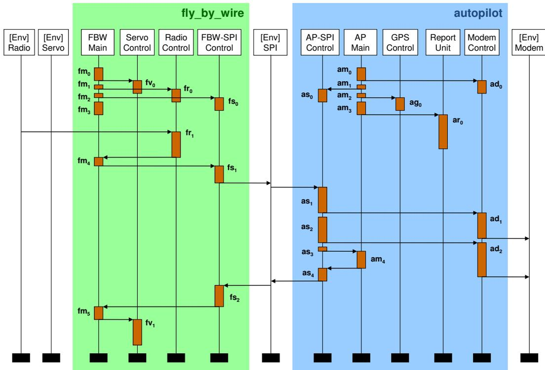
Figure 7.1: Message Sequence Chart model of the adapted UAV control application
